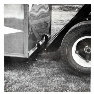
To pick up a loaded grain body, the driver aligns the truck just ahead of the filled body with the truck hoist fully raised. He hooks cables to long beams under the grain body, then returns to the cab to operate controls which winch the truck back against the rails at the front of the grain body. As the grain body begins to slide up the truck's long beams, he lowers the hoist.
