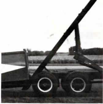
When the front of the body is about as high as the truck frame (photo below), he lowers the hoist until the angle of the hoist's long beams, and the truck body beams, is the same. He then winches the grain body aboard, allowing the truck to roll back freely under the body until the rear of the grain body leaves the ground. Entire loading or unloading operation takes less than 10 minutes.
