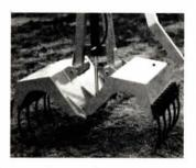
The spring steel tines on the bucket open up to 4 ft., 2 in. The height of the bucket and boom is 5 ft. 6 in. and it weighs about 600 lbs. It'll fit either 2 or 4WD tractors and loaders equipped for either hydraulic or manual tipping. The Eze Load sells for about \$1,500. The company is looking for a North American distributor.
