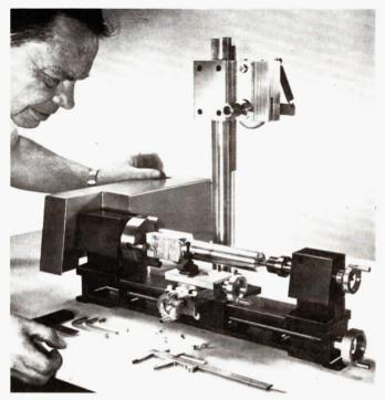
New Machinex 5 combines five functions — a lathe, drill press, vertical milling machine, grinder and polisher — into one unit. You can do cylindrical turning, facing, boring, drilling, reaming and other operations.
