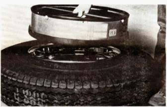
Bottom edge of Bead-Up and edge of rim and tire are painted with lubricant to create tight seal for seating the tire.
