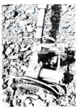
motor which rotates the threaded rod to push the disc out or pull it in.
