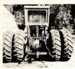
The Cummins engine ran too fast in the field so Carroll used a combine governor to slow it down, running the governor off the power steering drive belt.
