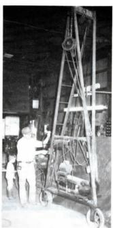
Lifting by the overhead carrier is controlled by a 3-speed Studebaker transmission that direct-drives an old Farmall F-20 steering gear. A cable spool is fitted to the steering gear. Cable runs from the spool up to the overhead lift carrier. The transmission is driven by electric motor. To control speed and direction of the lift cable, you simply change gears on the transmission.
