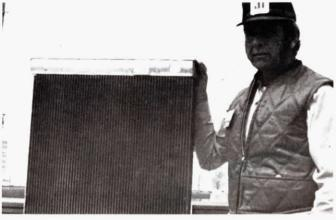
Bill Ernsting has developed what he calls his "feedlot special" radiator. It's designed for use in trucks used in and around feedlots, or silage or haying operations.
