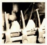
grinder. He cuts a curve into the end of the section that's 1/16 to 1/8 in. deep. "If you have rocky soil you should hollow it out less to avoid chipping." he notes.
