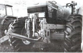
We're introducing a TwinLink front 3-pt. system for 4- and 6-cyl. Ford New Holland PowerStar tractors equipped with front wheel assist. All TwinLink systems are integrated with the tractor design ensuring that there is no interference with steering, tractor clearance, lights or routine maintenance accessability.
