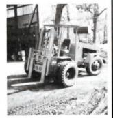
operate the mast. The pump is chaindriven off the engine crankshaft. The mast has four cylinders - one to raise it up or down, two to tip it forward or backward, and one to shift it from side to side. I use the bus's original power steering pump to provide hydraulic steering. The pump powers a hydraulic cylinder that's connected to a pair of tie rods that I welded onto the bus frame. A hydraulic cylinder is used to operate the brakes."
