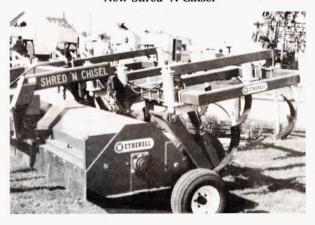
Wetherell's new Shred 'N Chisel is designed to shred corn stalks in the fall and bury them at the same time with the rearmounted chisel to prevent wind-blown trash and erosion.
