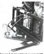
either use it at ground level, or swivel it 90 degrees and use it high up in the air as a trimmer. A single 4-in. dia. cylinder with a 20-in. stroke provides cutting power. It activates a large steel blade that pushes through the tree trunk or branch into a slotted set of gripper teeth.
