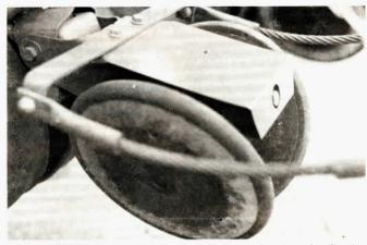
Couser's shield keeps clods and roots from plugging the firming wheels.
