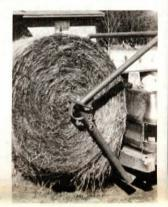
that one advantage of his design over commercial units is that you can leave the tailgate on the pickup and still pull a trailer even with the bale handler on. The rig can be removed in seconds by pulling a couple pins.
