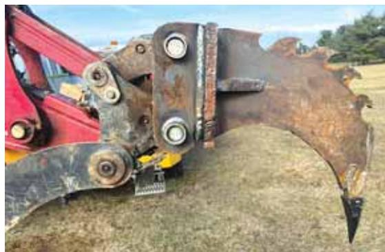
Sprouse built a ripper claw for his mini-excavator from an old grader blade.
