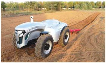
YTO 220-hp. cabless tractor has an operating error rate of less than one inch.
