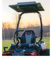
CoolTops have a built-in 12-volt electric fan that runs from the tractor or mower
