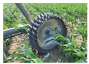
Tread design gives up to 55 percent reduction in rutting compared to conventional wheels.
