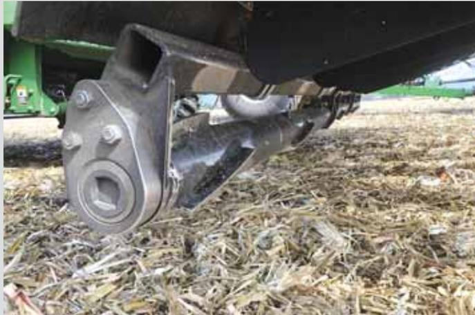
Devastator uses flat steel roller bars that knock over stalks and crimp them as the combine moves through the field.
