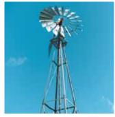
Windmill sizes range from 30 to 80 ft., with 6 to 16 ft. diameter wheels.
