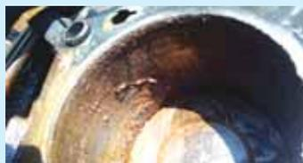
Peterson used lp gas to cool and shrink the piston enough to turn the engine over and free the rusty cylinder.
