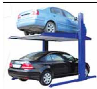
Two-post lifts save space but need a sturdy concrete floor of 4 to 5 in. thick for installation.
