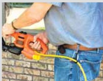
Larry Goodman, Ionia, Mich.: "I accidentally cut the cord while I was trimming shrubs with my electric hedge trimmer. While I was fixing the cord, I had the idea to hook a carabiner clip to my belt loop and run the extension cord through it. The cord moves easily and it's out of the way."
