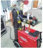
Welder Kaddy is 10 in. wide by 18 in. long and about 3 1/2 in. deep. It's made from 12-gauge steel and powder-coated. It and two earlier versions, including the prototype, find daily use in the Melius shon.
