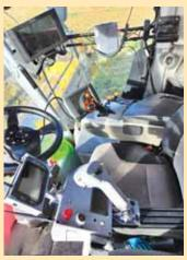
Combine cab with left hand joystick for tractor.
