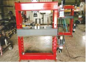
Variablespeed H-frame press cylinder can travel back and forth and slow or speed up as needed.
