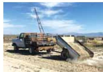
**"It works without any hydraulics or complicated mechanics. When the bed empties, it tips back and locks into place," says Hoard.**
