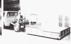
Truck platform remains parallel with the ground at all times as it's raised hydraulically into regular position for down the road travel.
