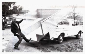
Two front-mounted springs pull the dump box back to transport position when empty.
