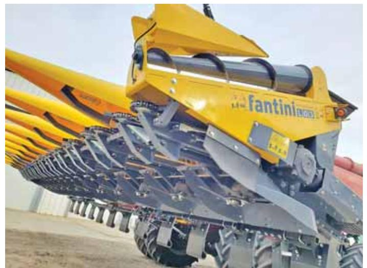
"The chopper placement lets it chop the stalk as it comes through the corn header. The stalk is sucked to the top of the rolls without beating the kernels off the cob," says Moran.
