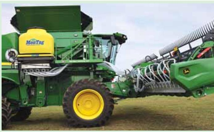
RBS Harvest Seeder mounted on soybean head.
