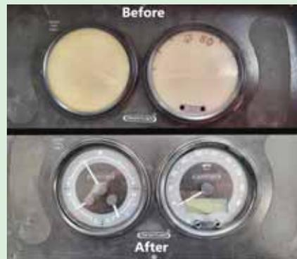
Control board was fixed, but lenses were cloudy, so replacement lenses were 3D printed.
