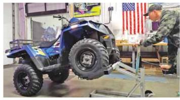
EZ Pro Lift has a 750-lb. front lifting capacity with a 25-in. lifting height. It handles tires as wide as  $10\ 1/2$  in. and up to 26 in. tall.
