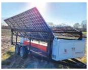
Solar powered trailers can provide power to remote locations or be used when regular power is out.
