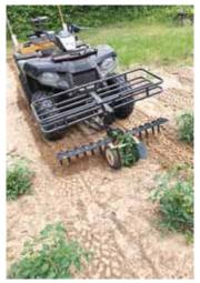
"I added mounts for a set of wheels from an old rototiller to the bar, giving the tines about a 1 1/2-in. depth. I also added galvanized aluminum shields inside the wheels to keep from running over plants," says Sieting.
