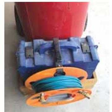
Strayer used some extra air chucks for an extension to make draining the tank easier. He also added a tool box and cord reel for hose storage.
