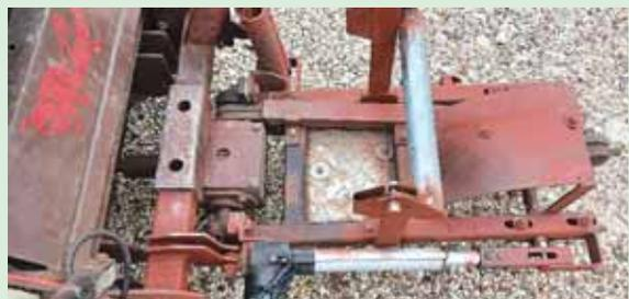
"I incorporated a 1-in. keyed shaft for the mower pto. The gearbox mounts to the pto shaft with a keyed coupler."
