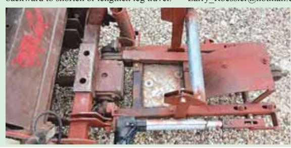
I incorporated a 1-in. keyed shaft for the mower pto. The gearbox mounts to the pto shaft with a keyed coupler."
