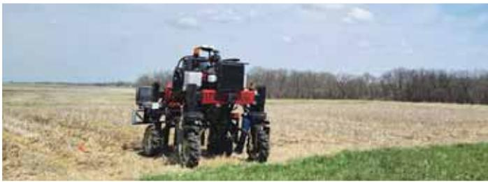
Flex-Ro has been working within test plots and has succeeded at planting corn and soybeans while moving at a pace of around 2 mph.
