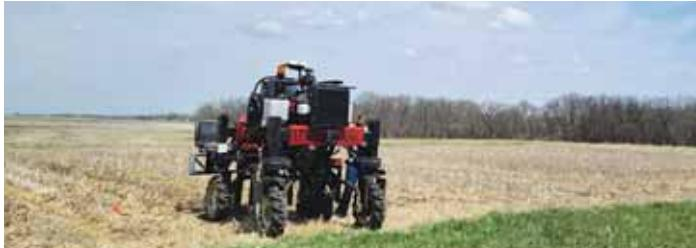
Flex-Ro has been working within test plots and has succeeded at planting corn and soybeans while moving at a pace of around 2 mph.
