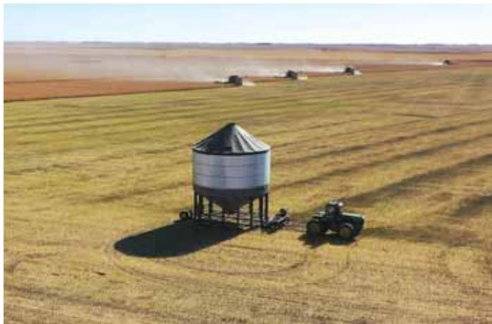
**Once pulled to the desired location, transit dollies lower the T-bin to the ground. The 8-ft. high roof with an 18-gauge seam-sealed roof tarp and 36-in. top opening is telescoped into place.**
