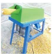
Operating at a speed of 2,800 rotations per minute, it takes about 3 to 5 seconds to thresh each ear of corn.
