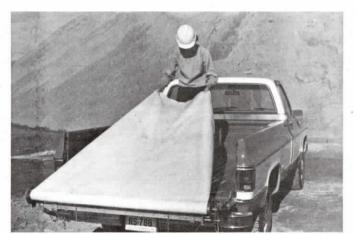
Super-tough slip sheet is rolled out on the pickup bed and the load (up to 3,000 lbs.) loaded on top of it. Rolled up unloading apron can be left in place between jobs.
