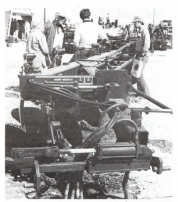
When driver changes cutting width "on the go", the hitching point also moves, providing automatic line-of-draft-adjustment.
