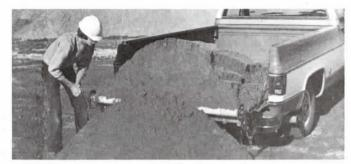
As slip sheet is wound up on the roller, it gently slides the load towards the tailgate and dumps it off slow and easy.
