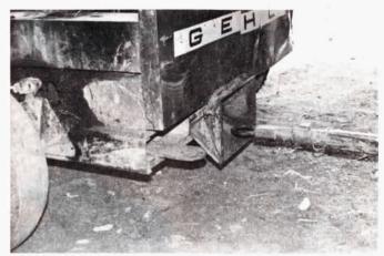
Koopman automatic hitch fits tractors, trucks, choppers, balers and other implements. Allows hitching, unhitching right from driver's
