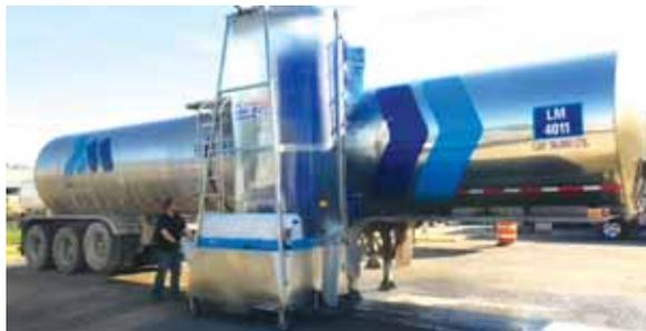
**Mobile wash units are an alternative to fixed bay washes using large brushes to clean around contours.**
