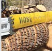
Lance B., via www.repurposedmaterialsinc.com: "I used 3-in. fire hose cut into sections to make protective sleeves for my chain saw bars."
