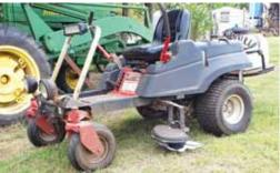
Krueger made an extension from 3-in. box tubing to mount the power head from an old DR trimmer head to the side of the zero-turn.
