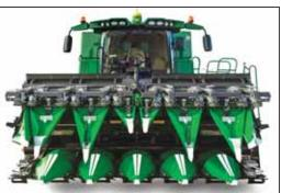
Folding option is unique to Drago as no hydraulics are used. Simple lever operation allows it to slide into place as connections are made.
