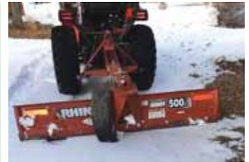
Edes slid an old tire over his snow blade and secured it with a rope to keep gravel from getting dug up by the blade.
