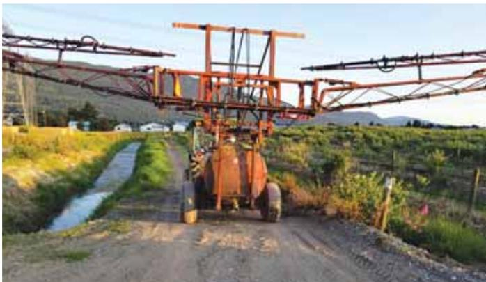
Dalton removed the short spray booms from the sprayer mast frame and mounted the new spray booms. No other changes were needed to the older sprayer.
