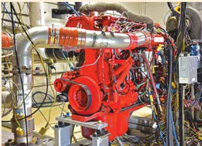
The ClearFlame technology involves increasing the temperature to make ethanol ignite as easily as diesel. It includes reengineering the fuel injection system for ethanol.
