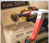
Crescent Tools (www.crescenttool.com; ph 866-907-9716): Have you heard about the Screw Biter screwdriver from Crescent Tools for removing damaged, corroded, or stripped screws. You simply align the Screw Biter bit with the screw head and strike the steel end cap of the spring-loaded handle. An internal mechanism uses that impact force to turn the screw 12 degrees, breaking it loose. A 2-piece set with flathead and Phillips bits sells for about \$25."
