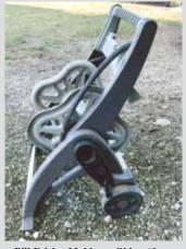
Bill Fricks, Muldrow, Okla: "I use a garden hose reel to wind up electric fence wire. I just disconnect the opposite end and start winding. If there are splices, I take the wire off the insulators and wind in one spot. The wire comes in easily. I have another rig for a 2-wire fence. I pick up hose reels for free when people leave them at dumpsters. Works very well."
