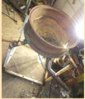
Isaac Voeller built a homemade forge out of an old wheel rim and exhaust tubing.
