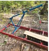
Come along attaches to 3-pt. boom to move logs onto sawmill.
