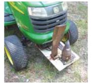
Front-mounted splitter runs off a chain drive mounted to a lawn tractor.
