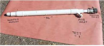
White has had the device tested by an independent lab. It tested the unit on tap water and raised DO by 137.5 percent.
