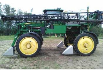
Crop protectors mount in front of lead axles and under sprayer frame and are easily
