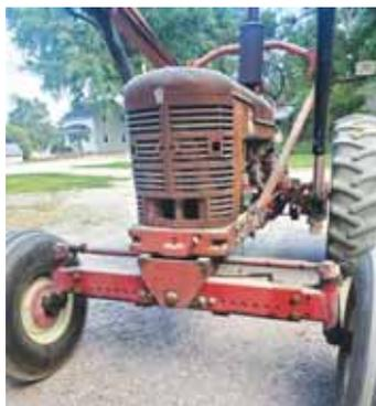
**Klahn removed the narrow front-end pedestal and fabricated a mount for the combine axle that fit in its place. He also removed the steering shaft and replaced the steering wheel on the throttle/steering wheel post with the steering wheel and motor from the 915.**
