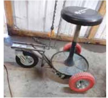
For the traveling chair, Brad added a frame and three 8-in. wheels, with the front one a multidirectional wheel.
