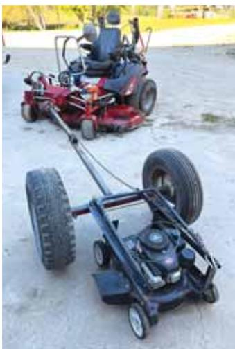
Hernke mounted a 20-in. push mower on a two-wheel cart with a long reach and uses it to mow around culverts and steep banks.
