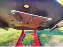
Cutting plate made of 3/4-in. thick Grade 50 steel with reinforcements on the blade mounts and center hub add strength to the skid steer-mounted Mega Mower X.
